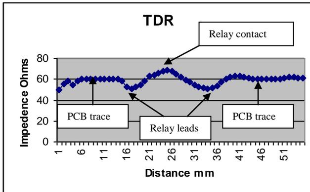
The relay package has a large impact upon the RF characteristics of the device. Surface Mount Device (SMD) packages offer better performance than through-hole packages. The leadless and axial packages offer the overall best performance and highest bandwidths. Figure 1 shows the insertion and return losses for a gullwing SMD relay. The performance of a similar device mounted in a leadless ceramic package is shown in figure 4.
