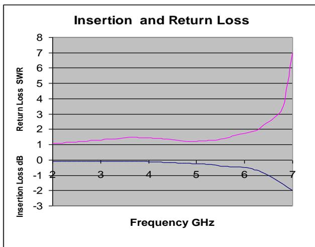
The  $-3$  dB roll-off points between the gullwing device shown in figure 1 and the SMD leadless device shown in figure 3 are approximately 7.5G Hz and 5.7G Hz. The rise times of the leadless SMD and the gullwing device are calculated at 47 picoseconds and 61 picoseconds respectively. This improved RF performance for the leadless device is generally due to the improved signal path through the relay.
